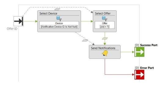
You can also select which are the users to be notified by using the dedicated "Device" class available in the Domain Model. This class stores information about the device on which the mobile application is installed and it is directly connected to the mobile application user. The device information are retrieved by the mobile application when the user logs in; in that moment the mobile
