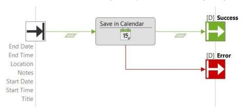
The behavior of the mobile application is to open up the device calendar showing to the user the form for creating a new event. The form is preloaded with the information you specified in the model and the user can decide whether to save the event or to cancel the operation. In both cases the user then goes back to your mobile application.
